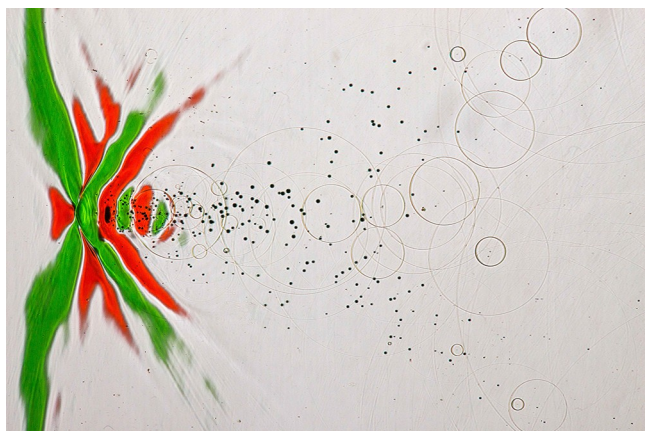
Figure 1. Shock wave pulse visualized by color-schlieren-optic. Shock waves are pressure waves traveling, e.g., through water as pressure distortions with a velocity of approx. 1500 m/s. Usually, the pressure distortions are not visible by the naked eye. A color optical schlieren apparatus [29] can visualize gradients of the pressure distortions, which are here displayed in red (pressure rise) and in green (pressure decline). The shock wave is traveling from right to left. The first small red triangle on the symmetry axis left depicts the area of rapid pressure rise. From the peak, the pressure decreases, displayed in green color until the minimum pressure is reached and is again raising (displayed in red). Several smaller reverberations with alternating pressures and according to pressure gradients are displayed further to the right. After the first minimum pressure (right rim of the first green line) a field of cavitation bubbles occurs. Some of the bubbles collapse already and radiate secondary spherical shock waves depicted by the circles at the right side of the frame. Shock waves like the one displayed are transmitted from outside the body through the intact skin into deeper target areas of the tissue, where they stimulate tissue interfaces or fragment body stones via the mechanism of momentum transfer.
